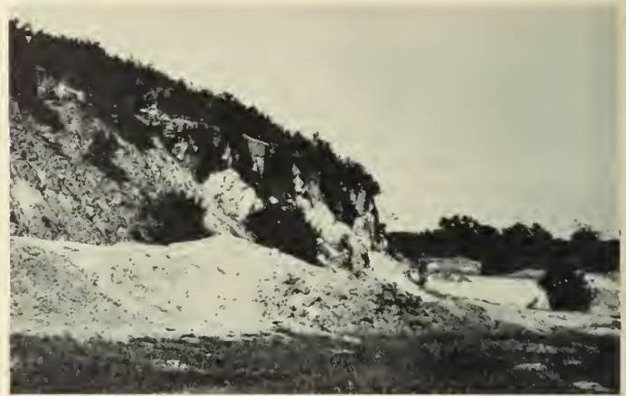
FIGURE 12. Woolford clay pit. White area in right center is Cheney Hill clay. Overburden is white, buff, and brown sandstone and conglomerate. The pit is now idle.
